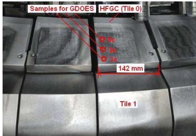
Fig.5 Tiles HFGC in JET wall
