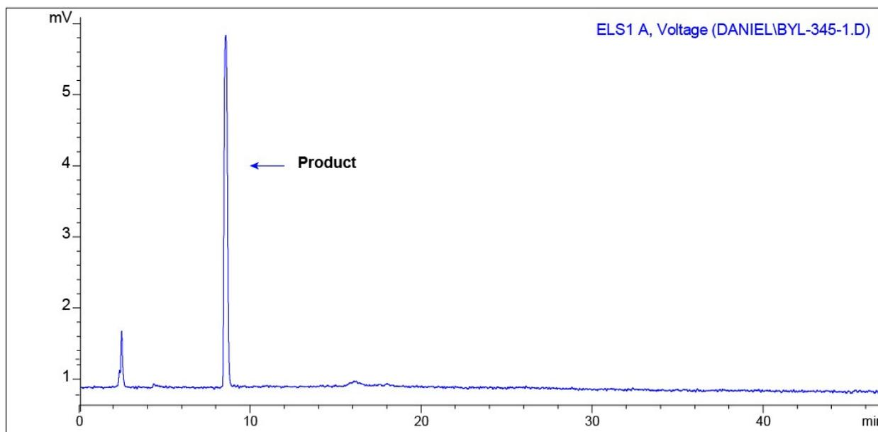
**Normal Phase HPLC analysis of compound 2.** The analysis was performed on a Agilent 1200 HPLC system using a YMC DIOL column (4,6 x 100 mm), a gradient of ethyl acetate in n-hexane from 10 to 90 % in 30 min, and 1 ml/min flow rate. The detection of the compounds was performed using an ELSD detector.
