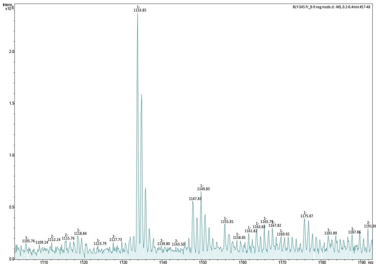
ESI- MS Analysis of Compound 2 carried out on a Bruker amaZon Speed ETD mass spectrometer in negative mode. (M+OH)<sup>-</sup> MS<sub>calculated</sub> 1133.66, MS<sub>found</sub> 1133.85.
