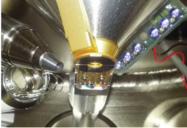
Figure 2.7: Photo of the vacuum chamber of a Zeiss Supra 40 SEM (Oberkochen, Germany). The backscattered electron detector is placed in a ring design below the pole piece while the energy dispersive X-ray detector and secondary electron detector are mounted laterally.
