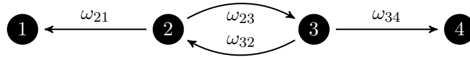
Figure 2.2: Markov process with absorbing states. States 1 and 4 are absorbing states, whereas states 2 and 3 are transient states. The rate of transitions from state i to state j is denoted by \omega_{ij} .
