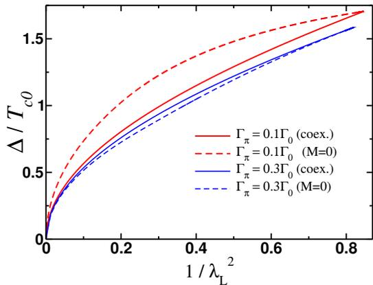
FIG. 6: (Color online) Plot of  $\lambda_L^{-2}$  on  $\Delta$  across the phase diagram at  $T = 0.01T_{c0}$ . Remarkably, the position of the line for the purely superconducting state depends on the strength of the interband scattering rate. This is expected as the superconducting order parameter is strongly suppressed for higher values of  $\Gamma_\pi/\Gamma_0$ .
