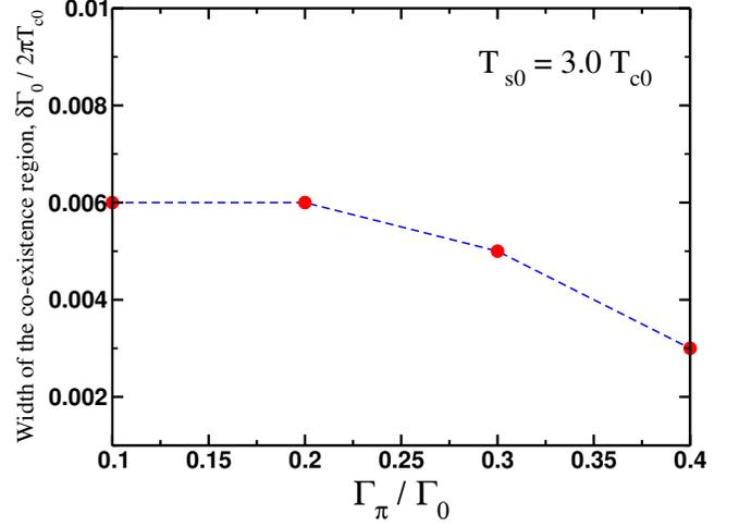
FIG. 2: (Color online) Width of the coexistence region  $(\Gamma_0^{(sdw)} - \Gamma_0^{(sc)})/2\pi T_{c0}$  is shown as function of  $\Gamma_\pi/\Gamma_0$ . The data points are found from the solution of Eqns. (18) and (17) at zero temperature. The plot is obtained assuming  $T_{s0} = 3T_{c0}$ .
