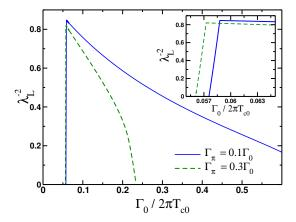
FIG. 4: (Color online) Inverse square of the London penetration depth (dimensionless units) as a function of intraband scattering rate  $\Gamma_0$  evaluated at  $T = 0.01T_{c0}$ . In the coexistence region  $\lambda_L^{-2}$  grows linearly with  $\Delta$  in contrast with the clean case where  $\lambda_L^{-2} \sim \Delta^2$ , Eq. (31).
