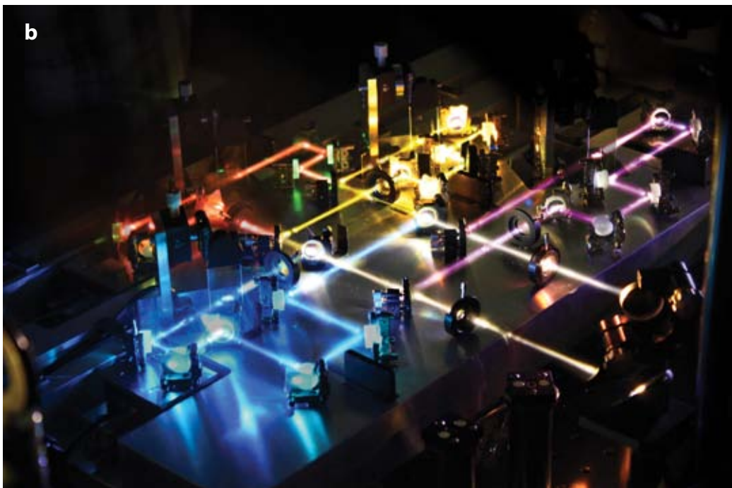
Figure 2.5: Second generation light field synthesizer. a , Schematic representation of the synthesizer. DBS: Dichroic beam splitters; CM: Chirped mirrors. Pulses in each channels are compressed and their temporal profiles are shown accordingly (same color codes). b , Photograph (perspective view) of this synthesizer in operation. Adapted from [17].
