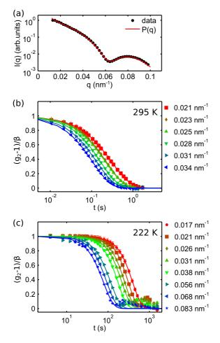
FIG. 1. (Color online) (a) Plot of I(q) from the studied sample and particle form factor fit P(q). (b) and (c) Intensity autocorrelation functions  $g_2$  at different q values for (b) T=295 K and (c) T=222 K. Solid lines are fits with the KWW function (1). For 222 K additional contributions at longer time scales can be observed. In both cases the time axes cover three orders of magnitude.
