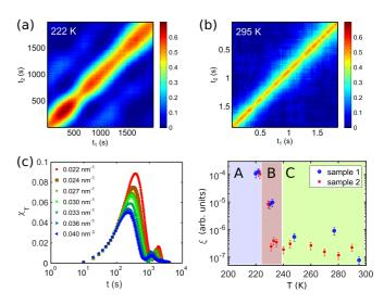
FIG. 4. (Color online) Two time correlation functions  $C_I$  for (a) 222 K and (b) 295 K at  $q = 0.023 \text{ nm}^{-1}$ . (c) Plot of  $\chi_T$  for 222 K. (d) Plot of  $\xi(T)$  for two samples of slightly different volume fraction of tracer particles. The regions identified in Fig. 3 are indicated by A, B, and C and different background colors.
