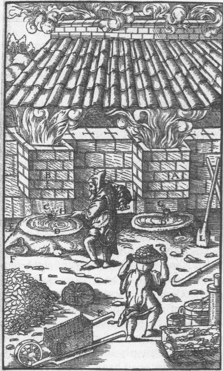
A, B—TWO FURNACES. C—TAP-HOLES OF FURNACES. D—FOREHEARTH. E—THREE TAP-HOLES. F—DIPPING-POTS. G—AT THE ONE FURNACE STANDS THE SMELTER CARRYING A WICKER BASKET FULL OF CHARCOAL. AT THE OTHER FURNACE STANDS A SMELTER WHO WITH THE THIRD HOODED BAR BREAKS AWAY THE MATERIAL WHICH HAS FROZEN THE TAP-HOLE OF THE FURNACE. H—HOOKED BAR. I—HEAP OF CHARCOAL. K—BARROW ON WHICH IS A BOX MADE OF WICKER WORK IN WHICH THE COALS ARE MEASURED. L—IRON SPADE.
