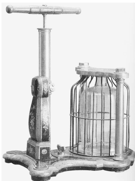
Jean Antoine Nollet's vacuum pump apparatus with protective cage (from Lewis Pyenson and Jean-François Gauvin, eds., The Art of Teaching Physics, p. 140).
