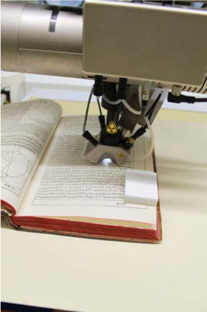
Figure 1.5: X-ray fluorescence analysis of the ink used in underlinings found in a copy of Guidobaldo's mechanics. The underlinings were written with an iron gall ink from the period. They concentrate on the foundational aspects of Guidobaldo's approach, his comments on Aristotle, and the critique of his adversaries.
