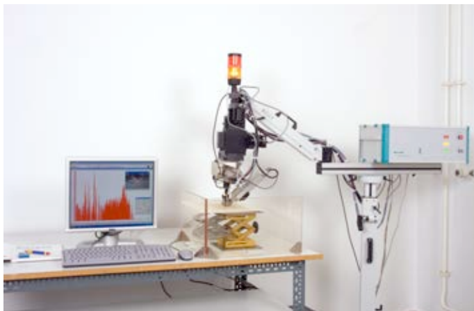
Figure 11.1: Mobile XRF spectrometer.
