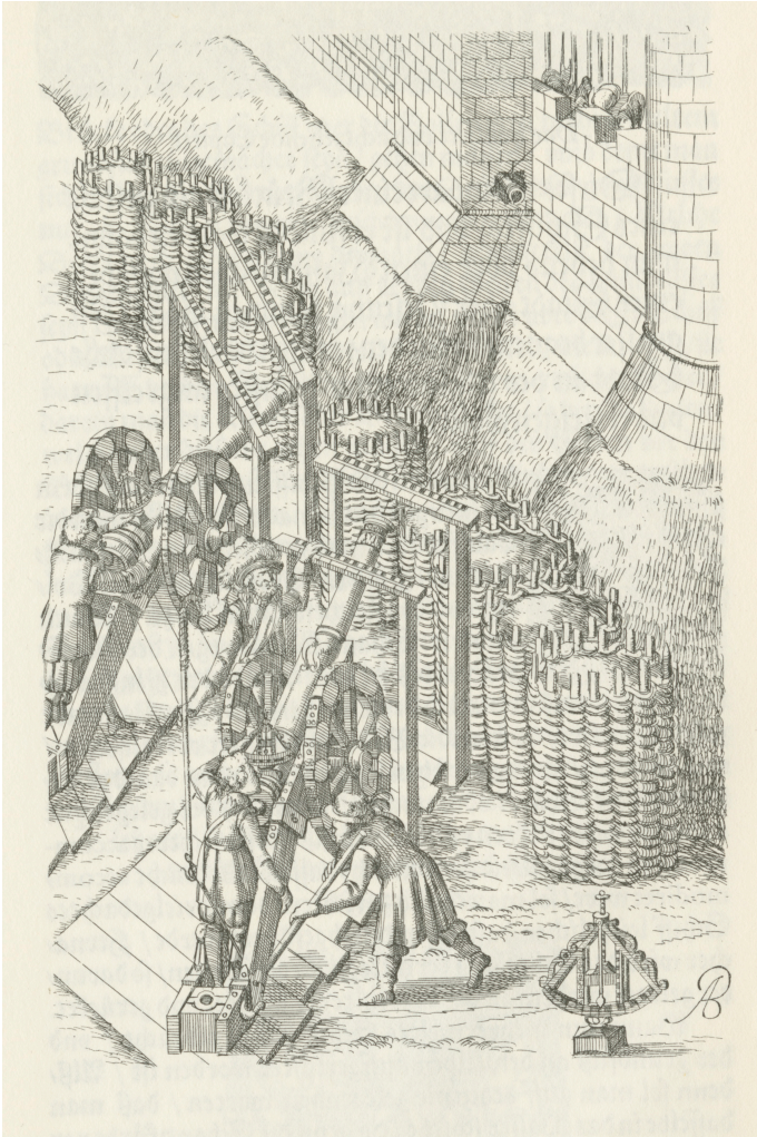
Figure 5.1: Drawing illustrating how, during the sixteenth century, artillery was used by targeting points in the front of the fortress whose distance was measured by means of a straight line. These replaced the buildings located inside the fortress as targets to be destroyed by means of high shots over the walls. From the German edition of Ramelli 1588 published in 1620.
