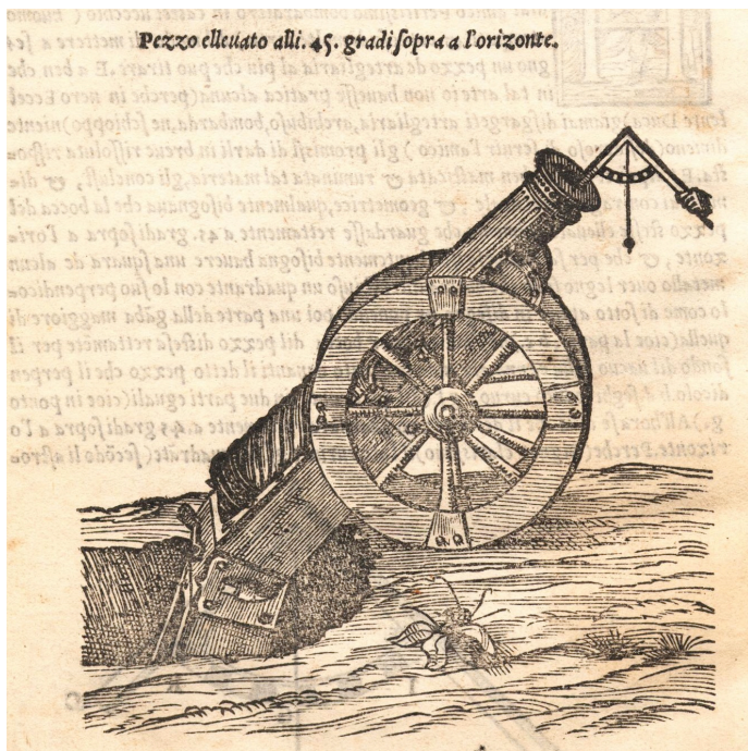
Figure 2.1: Representation of a cannon positioned at a 45-degree angle of elevation as verified by means of the bombardier's quadrant. From Tartaglia 1558, epistle, second folio (unnumbered), verso.
