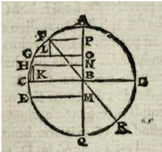
Figure 3.9: According to Cardano, there are three ways to determine positional heaviness. The positional heaviness at point F , for instance, may be determined by the horizontal FP , by the vertical FL , or by the angle QBF .
