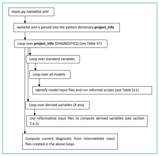
Figure 2 ESMValTool control flow.
