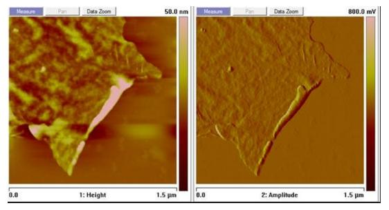
**Figure SI 1:** Typical AFM measurement of a single, rolled up sheet transferred to a silicon surface illustrating the large scale homogeneity, transferability and and the mechanical intactness of each single carbon nanosheet. Left: Height view; right: amplitude view.
