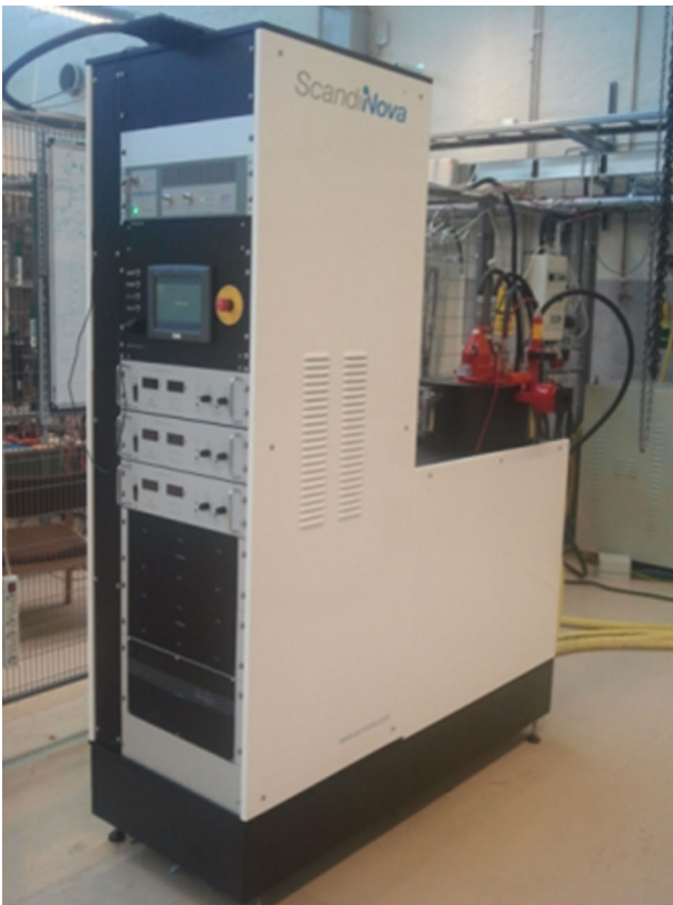
FIG. 24. Photograph of the compact rf transmitter that provides all power to photoinjector and linac.
