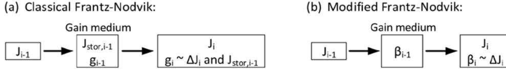
Fig. 2. Comparison of (a) the classical and (b) the modified FN equations. While the classical equations define and utilize a stored fluence  $J_{stor}$  the modified equations circumvent this expression by using the inverted fraction  $\beta$ .
