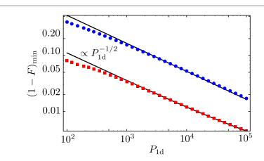
**Figure 6.** Scaling behavior of the minimal infidelity for the Pauli-X (red squares) and controlled-(-Z) gates (blue circles) with the same parameters as in figures 3(e) and (f). The scaling fits well with the scaling  $P_{1D}^{-1/2}$  (black line) for large enough values of the Purcell factor  $P_{1D}$ . For the phase shift gate the infidelity is arbitrarily close to 0 in the ideal case.
