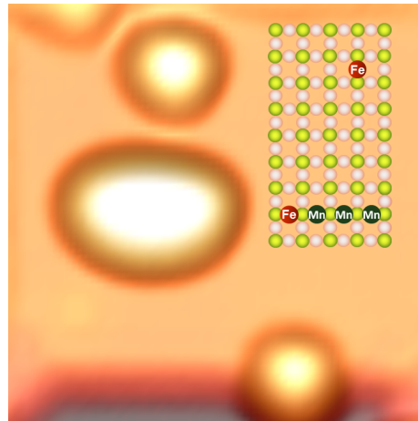
FIG. 1. Constant current STM image of a FeMn 3 chain assembled on a Cu 2 N layer and atomic scheme (on the right of the figure) that can be inferred from the position of the upper-right Fe atom and manipulation with the STM tip. The STM image was scanned at 10 mV and 100 pA. The scanned area is 6 \times 6 nm 2 . The transition metal atoms were always placed ontop of a Cu atom between two nitrogen atoms. The topography was processed with WSXM 25 .
