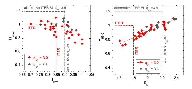
FIG. 10.: Normalized confinement  $H_{98y2}$  vs. density  $f_{GW}$  (left) and pressure  $\beta_N$  (right) for operation at  $q_{95} = 3$  (red) and  $q_{95} = 3.6$  (grey) in AUG-W (high  $\delta$ ). Target values for the ITER BL scenario and the alternative ITER BL scenario are indicated by red and grey broken lines, respectively.
