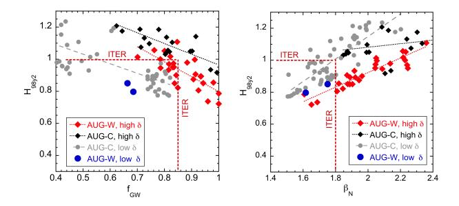
FIG. 9.: Normalized confinement  $H_{98y2}$  vs. density  $f_{GW}$  (left) and pressure  $\beta_N$  (right) for  $D_2$  stationary operation at  $q_{95} = 3$  in AUG-W and AUG-C at low and high triangularity. Parameters varied are gas puffing rate and heating power. Target values for the ITER BL scenario are indicated by red lines.
