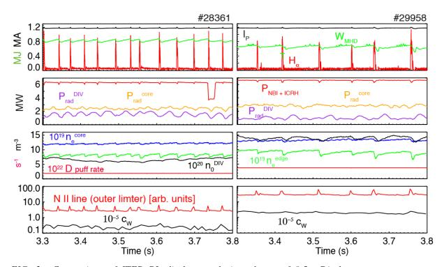
FIG. 2.: Comparison of ITER BL discharges during phases of 0.5s. Discharge parameters are identical except gas puff and 'freshness' of boronization. While the discharge on the left (#28361) was conducted 1 day after a boronization, the one on the right (#29958) was done 21 days after a boronization. Different gas puff levels  $1.9 \cdot 10^{22}$  and  $3.8 \cdot 10^{22}$  atoms/s were necessary to reach stationarity for discharges #28361 and #29958, respectively.
