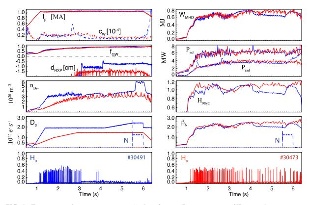
FIG. 6.: Time traces of various parameters (radiated power  $P_{rad}$ , separation of X-points  $d_{RXP}$ , nitrogen puff rate N) for two  $q_{95}=3.6$  discharges (#30491 with a type-II ELM phase, blue;) with different closeness ( $d_{RXP}$ ) to double-null configuration. For both discharges the toroidal field  $B_t = 2T$ , the applied heating power (NBI + ICRH) as well as the triangularity are the same.
