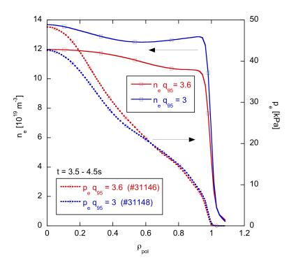
FIG. 4.: Radial profiles of electron density  $n_e$  and electron pressure  $p_e$  for the discharges of fig. 2 at  $q_{95}=3$  (#31148, blue) and  $q_{95}=3.6$  (#31146, red) averaged from 3.5s to 4.5s.
