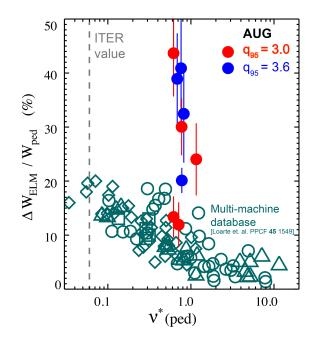
FIG. 5.: Energy loss of Type-I ELMs normalized to the pedestal stored energy vs. collisionality of the pedestal (value for ITER indicated by broken vertical line). Values for the two AUG scenarios at  $q_{95}=3.0$  and  $q_{95}=3.6$  are compared to a multi-machine scaling [9].
