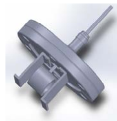
FIG.1. CAD drawing of the modified-PDX gauge in use on NSTX-U
