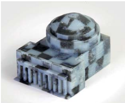
Figure 1: 3D printed model of a building with prescribed texture and subsurface scattering properties.
