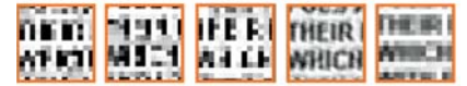
Apparent resolution enhancement for moving images: We optimize individual frames (1-3, from bottom left) so that they appear more detailed (ours, frame 4) on a human retina than conventional solutions (bottom right).
