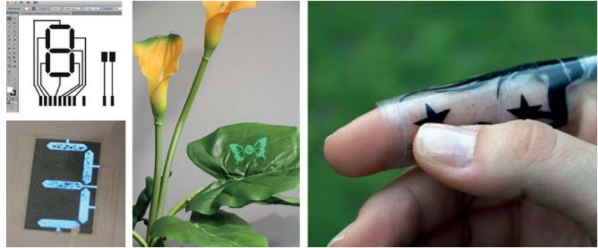
Our techniques allow to transform a digital vector graphics ( left ) into a functional, custom touch display for embedded user interfaces ( center ) and into a stretchable sensor for on-body input ( right ).
