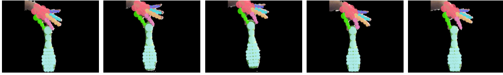
Figure 8.5. Subset of tracked frames on the dataset of [38]. Our method can handle objects with varying sizes, colors, and different hand dimensions . Here we show how even a complex shape like a bowling pin can be approximated using only a few tens of Gaussians
