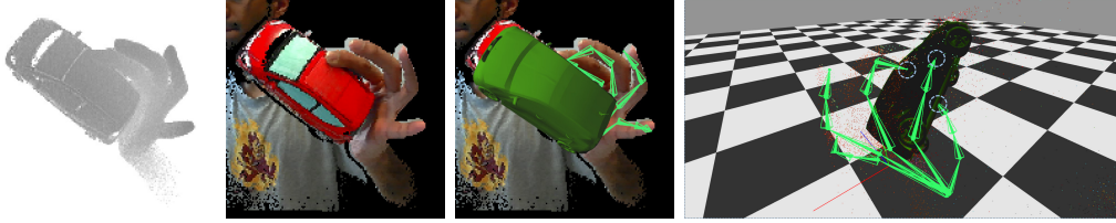
Figure A.2. We are able to track complex shapes like a toy car. Our contact points term (contacts are circled in blue) makes fingers hold the car even in the presence of severe occlusion.
