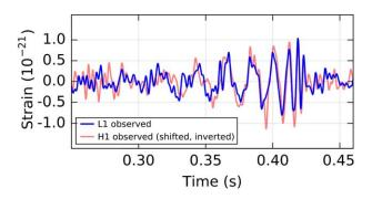
Figure 1 The instrumental strain data in the Livingston detector (blue) and Hanford detector (red), as shown in Figure 1 of [1]. Both have been bandpass- and notch-filtered. The Hanford strain has been shifted back in time by 6.9 ms and inverted. Times shown are relative to 09:50:45 Coordinated Universal Time (UTC) on September 14, 2015.
