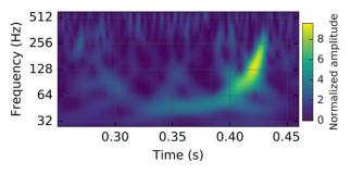
**Figure 2** A representation of the strain-data as a time-frequency plot (taken from [1]), where the increase in signal frequency ("chirp") can be traced over time.
