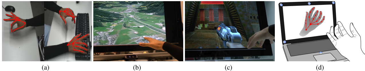
Figure 1. (a) FullHand can track one or both hands with all fingers. (b, c) FullHand enables free-hand interactions for many applications such as virtual globes and first-person shooters. (d) We envision miniature multi-camera setups for hand tracking in the future. The blue cylinders represent cameras.
