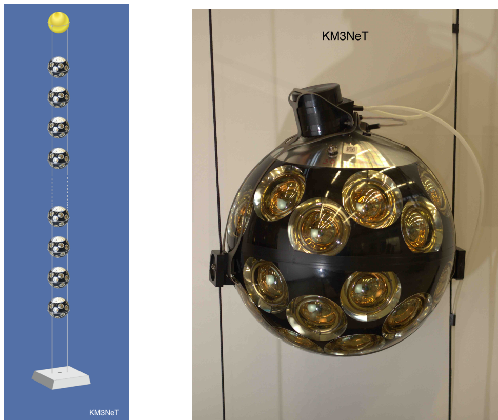
Figure 8: The detection string (left) and the breakout box and the fixation of the DOM on the two parallel Dyneema® ropes (right).
