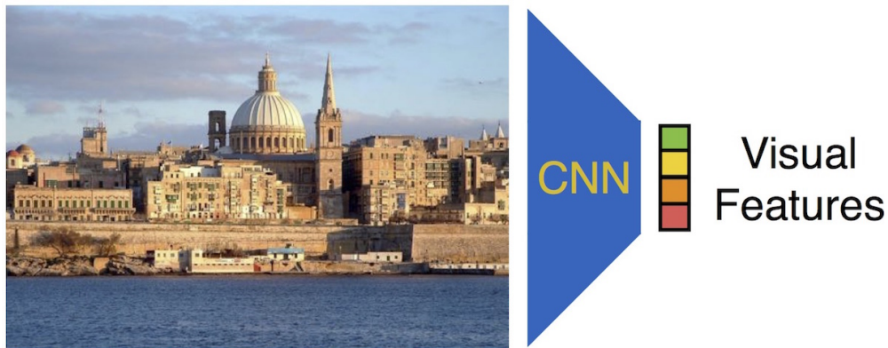
Figure 6: Features extractor. Neural responses of some layer to the visual input are considered as features.
