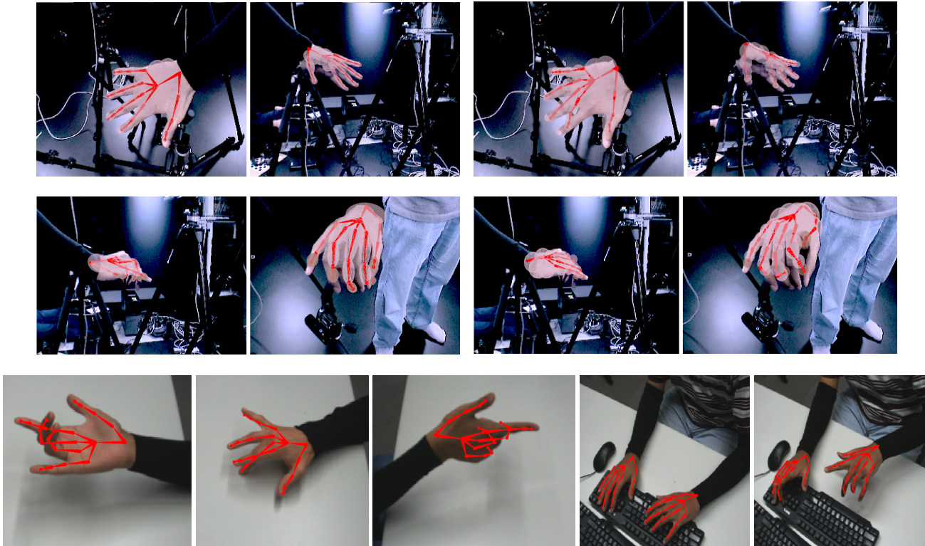
Figure 7. First Two Rows: Comparison of SAG (left) and SoG (right) for two frames in the Dexter 1 dataset. In the first row, SAG covers the hand much better during a fast motion of the hand in spite of using fewer primitives. In the second row, a challenging motion is performed for which SAG performs better. Bottom Row: Realtime tracking results for one hand with different actors, and two hands. Please see supplementary video for results from hand + object tracking.
