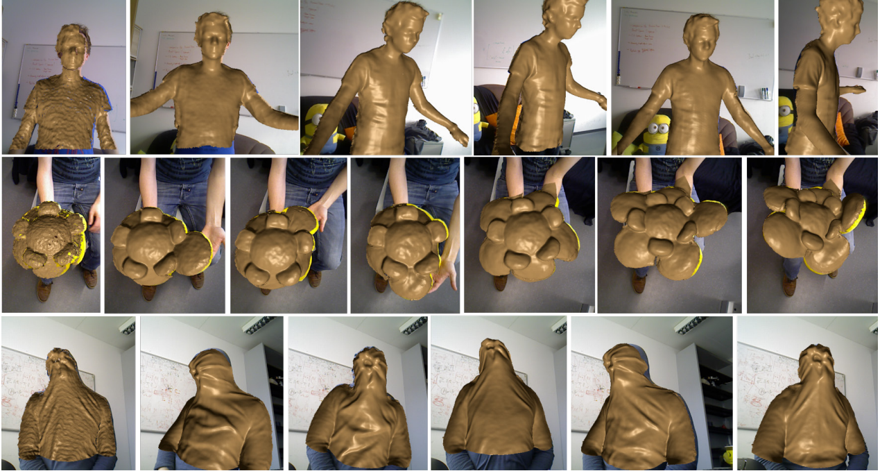
Fig. 3: A variety of non-rigid scenes reconstructed with our approach at real-time rates: UPPER BODY, SUNFLOWER, and HOODIE (top to bottom)
