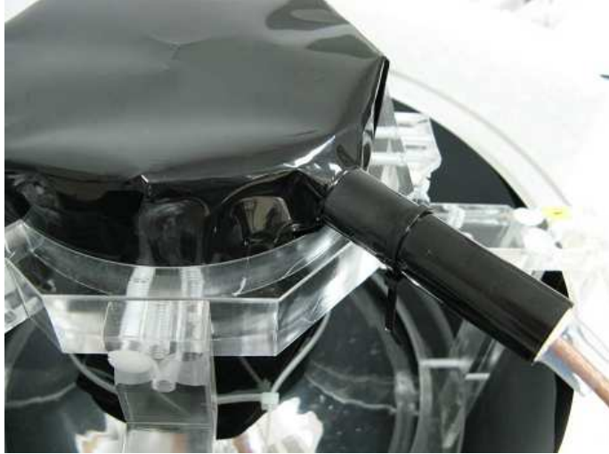
Figure 23. PMT base covered with black sheet as made for the near detector.
