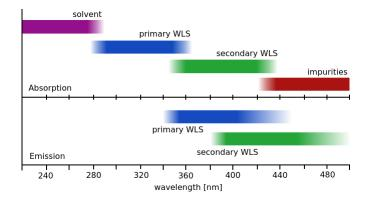
Figure 2: The plot shows for each scintillator component the wavelength region for which its own absorbance is dominating in the liquid. In addition the typical wavelength ranges for scintillator emission is shown for the case of just a primary or including a secondary wavelength shifter.
