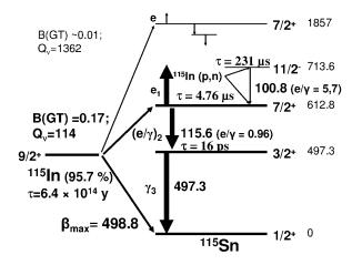
Figure 5: The term scheme of the <sup>115</sup>In-system is shown. Energies are given in keV. The energy threshold for the neutrino reaction is only 114 keV. In the reaction an excited state of <sup>115</sup>Sn is populated which has a lifetime of 4.76 $\mu$ s and decays to the ground state under gamma emission.
