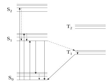
Figure 1: The energy levels of singlet (S) and triplet (T) states with the corresponding vibrational levels are shown for a fluorescent molecule. Solid arrows mark transitions leading to fluorescence or phosphorescence radiation whereas dotted arrows represent radiationless transitions.
