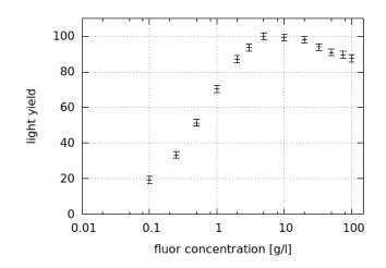
Figure 4: Relative light yield of a scintillator with methoxybenzene as solvent and increasing BPO concentration. The values are normalized to the highest light yield measured at 5 q/l.
