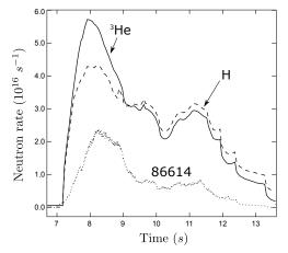
Figure 1: Neutron production rate (DD) for NBI+RF with a minority concentration of 4% in a deuterium plasma.
