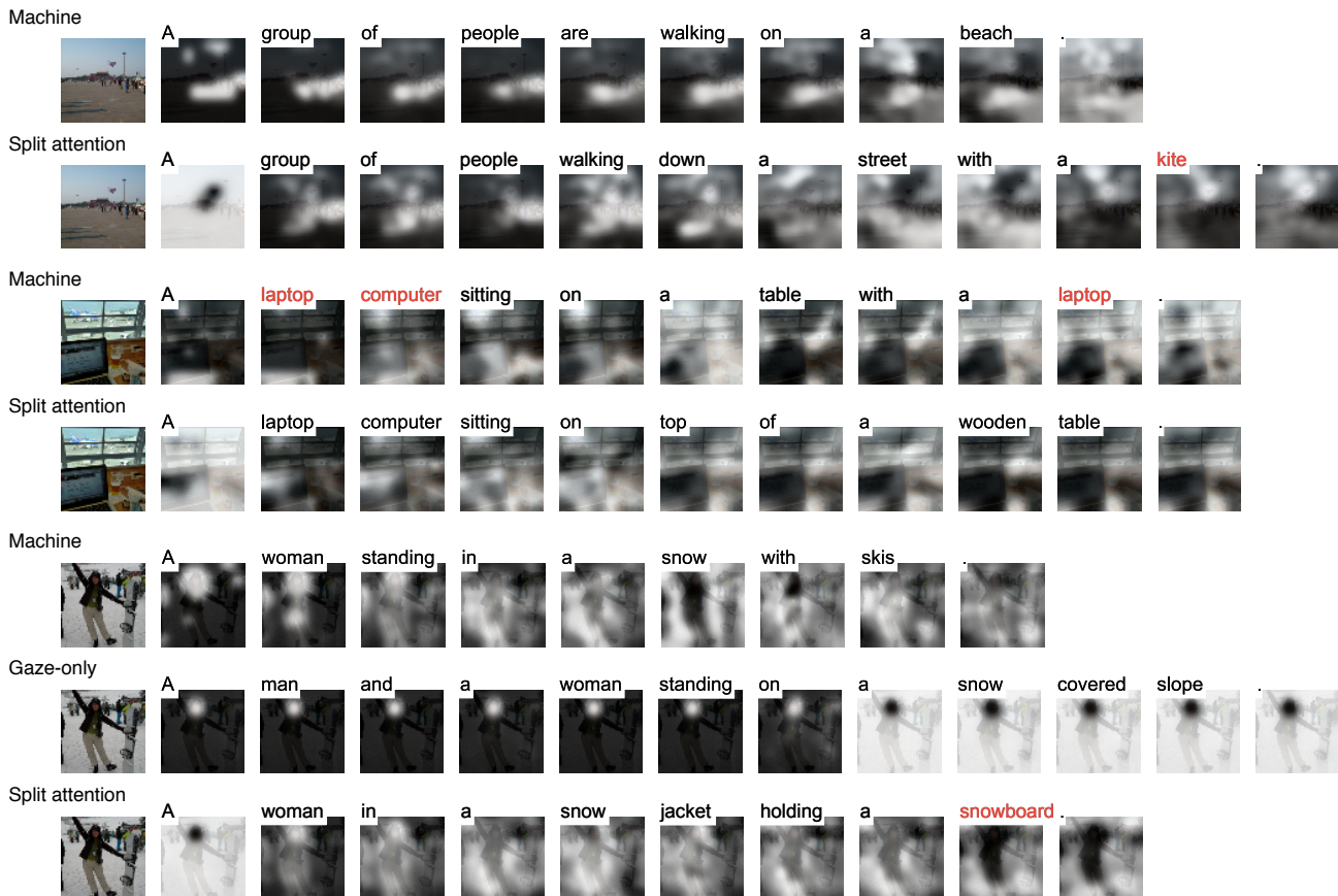
Fig. 5. Sample images, the machine attention map at each step as well as the corresponding output words for the baseline and gaze-assisted models. The first example illustrates the case where the proposed model finds small but important objects ( kite ) in the scene. It also helps to suppress the repetition of object description in cluttered scenes ( laptop in the second example). The proposed split attention model can also describe objects without strong fixation, such as snowboard in the third example. See the supplementary material for more examples.
