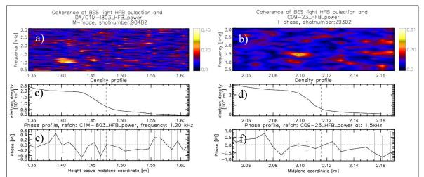
Figure 4.: M-mode (a) and I-phase (b) coherence of the HFB power modulation of the magnetics and the HFB pulsation of the BES light emission; M-mode (c) and I-phase (d) averaged density profile; M-mode (e) and I-phase (f) phase profile at the relevant frequency range relative to the HFB pulsation of the magnetics. Vertical dashed line indicates the LCFS position, horizontal dotted line shows the phase of the reference signal (0 phase line).
