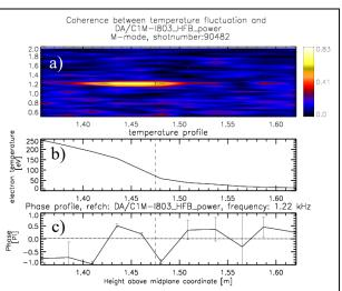
Figure 3.: M-mode temperature LFO characterization: coherence of the HFB power modulation of the magnetics and the LFO of the electron temperature (a); averaged temperature profile (b); phase profile at the relevant frequency range relative to the HFB pulsation of the magnetics (c). Vertical dashed line indicates the LCFS position, horizontal dotted line shows the phase of the reference signal (0 phase line).
