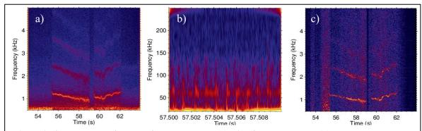
Figure 1.: Spectrogram of  $B_{pol}$  low frequency range (a), high frequency range (b) and  $B_{pol}$  HFB power modulation (c). (JET, shot 90482, Mirnov coil: C1M-I803)
