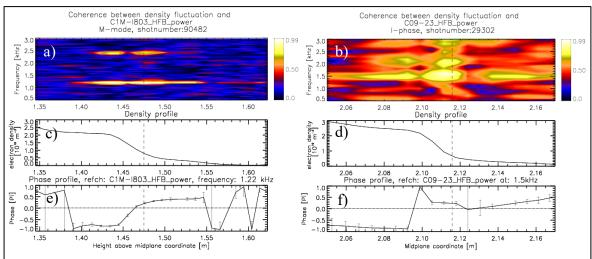
Figure 2.: M-mode (a) and I-phase (b) coherence of the HFB power modulation of the magnetics and the LFO of the electron density; M-mode (c) and I-phase (d) averaged density profile; M-mode (e) and I-phase (f) phase profile at the relevant frequency range relative to the HFB pulsation of the magnetics. Vertical dashed line indicates the LCFS position, horizontal dotted line shows the phase of the reference signal (0 phase line).
