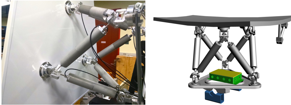
Figure 3: Left: Stewart platform holding a P1 panel. Right: CAD model of the final assembly of a mirror panel module, including mirror panel, Stewart platform, controller board, mounting triangle and one edge sensor (far right).
