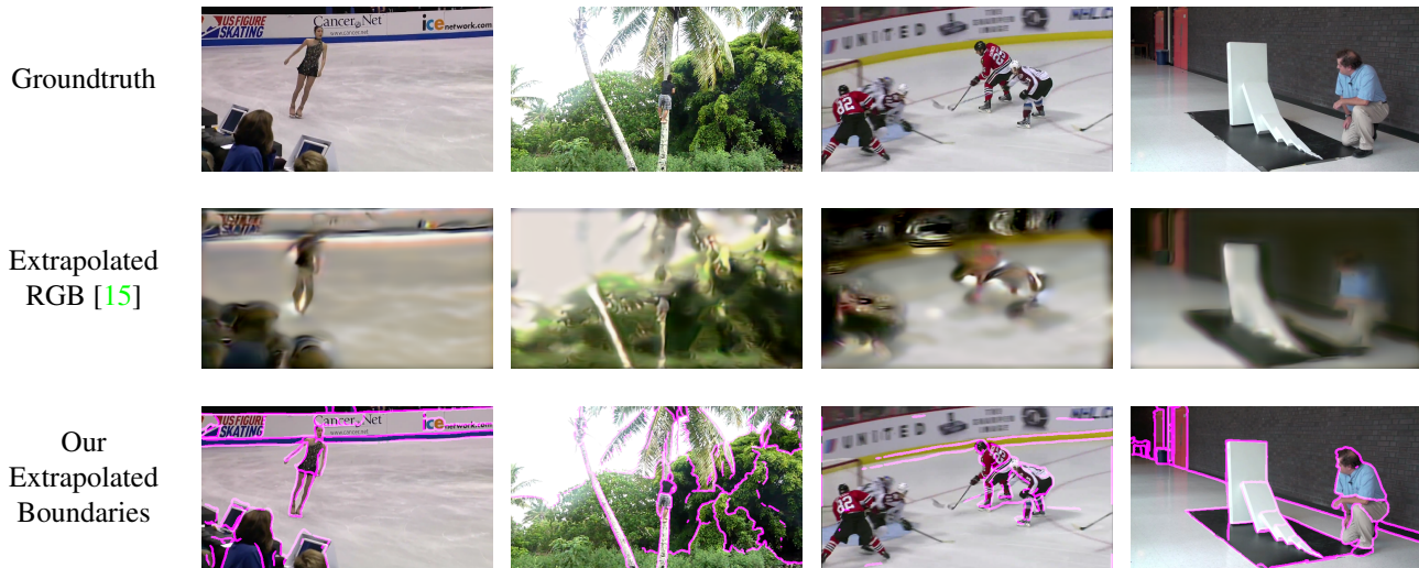
Figure 1: We predict the future of videos. (first row): the true future frame for t + 4 . (second row): RGB extrapolation of [15] which gets blurry quickly. (third row): our boundary extrapolation overlaid on the unobserved, true future frame, which outlines the boundaries precisely and enables long term prediction.
