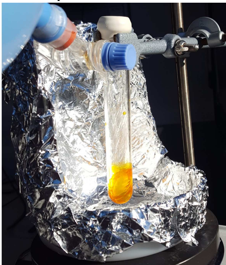
Figure S2. Typical setup for sunlight reactions.
