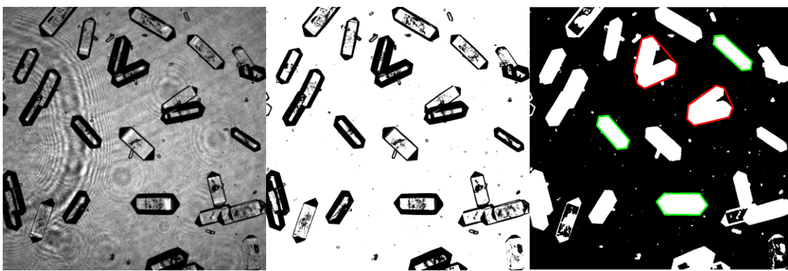
Fig. 4: Image processing of an exemplary chosen image acquired by the online microscopy. From left to right: Original image, background removal, binarization and single crystal identification.
