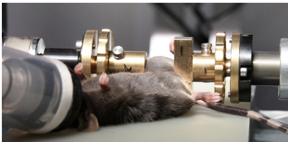
Figure 12: Photograph of a 10 week old C57BL/6J mouse undergoing in vivo loading of the left tibia.
