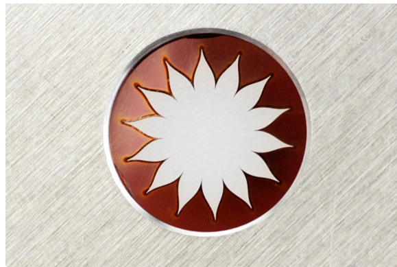
Figure 4. Photograph of the apodized aperture in aluminium mount. The bore in the aluminium mount has a diameter of 8 mm.
