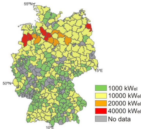
**Figure 4.2:** Maximum biogas plant capacity in the German districts in 2007 (adapted from *Scholwin et al.* [2008])
