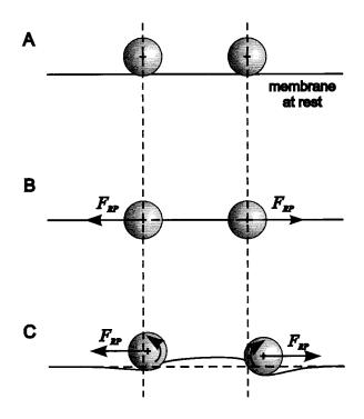
FIGURE 12 Scheme of the two-particle flat membrane geometry. (*A*) Unperturbed state with particles penetrating a small amount. (*B*) Particles with penetration d = 0. (*C*) A tentative representation of the out-of-plane deformation induced by the radiation pressure forces.
