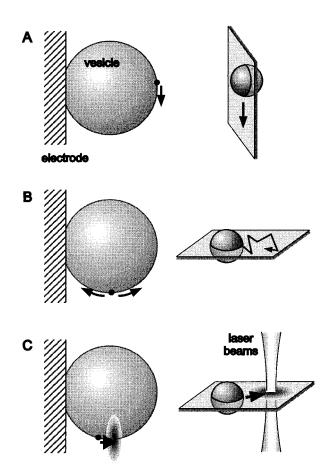
FIGURE 2 Schematic illustrations representing three different approaches to measurement of the mobility of a particle bound to a membrane. (A) Gravity-driven sedimentation. (B) Brownian motion at the bottom of the vesicle. (C) Optical trapping kinetics (the sketch is exaggerated in terms of distances).
