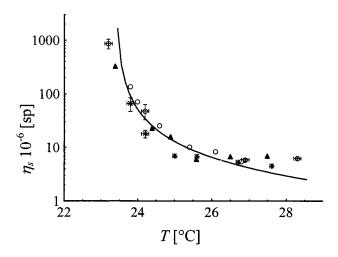
FIGURE 9 Temperature dependence of the shear surface viscosity,  $\eta_{\rm s}$ , obtained from sedimentation experimental data for three systems: a=2.64  $\mu{\rm m}$ , R=30.4  $\mu{\rm m}$ , d=-0.8 ( $\triangle$ ); a=2.7  $\mu{\rm m}$ , R=46.4  $\mu{\rm m}$ , d=-0.9 ( $\bigcirc$ ); a=2.72  $\mu{\rm m}$ , R=30.5  $\mu{\rm m}$ , d=0.1 (\*). The solid curve shows the fit by:  $\eta_{\rm s}=25\times 10^{-6}|T-23.4|^{-1.4}$  sp.
