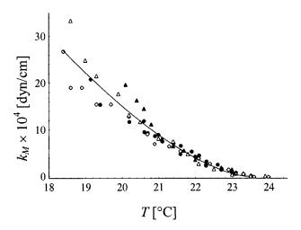
FIGURE 10 The measured membrane effective stiffness,  $k_{\rm M}$ , plotted as a function of the temperature. The different sets of symbols correspond to different temperature scans. Filled and empty symbols correspond to two individual particle-vesicle systems; for all particles  $a \approx 5.3~\mu {\rm m}, d \cong -0.8a$ . The solid curve shows the fit by  $k_{\rm M} = 2.4 \times 10^{-4} |T-23.4|^{1.5}$  dyn/cm.
