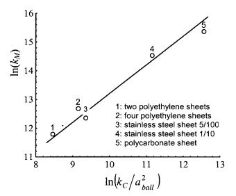
FIGURE 15 Test of the  $k_{\rm M}=Ck_{\rm C}/a^2$  relation. Measurements were performed on sheets of different materials, as indicated.
