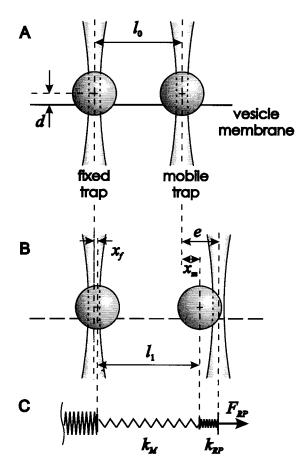
FIGURE 5 Experimental steps in the static elasticity experiment.  $d = R - \tilde{R}$  indicates the particle penetration depth (d is positive when the particle center is external to the membrane surface). (A) Initial position of particles. (B) Mobile trap displacement. (C) "Three-spring" model.
