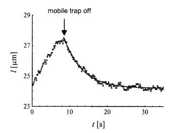
FIGURE 11 A dynamic elasticity experiment performed at  $T=19^{\circ}$ C. The points represent the measured interparticle distance, l, and the solid curve is an exponential fit following Eq. 11 ( $\tau_r=5$  s) to the relaxation branch of the trace.
