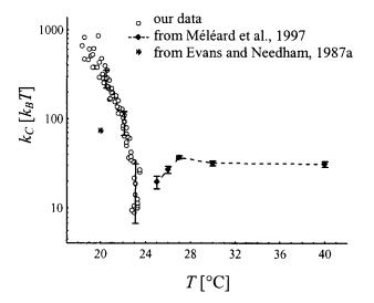
FIGURE 13 Thermal behavior of the gel-state membrane curvature modulus.  $\bigcirc$ , The values of  $k_{\rm C}$  were deduced from those of  $k_{\rm M}$  according to Eq. 12.  $\blacklozenge$ , Values of  $k_{\rm C}$  for fluid DMPC vesicles, taken from Méléard et al. (1997). \*, Single result on  $k_{\rm C}$  at  $T=20\,^{\circ}{\rm C}$ , taken from Evans and Needham (1987a).
