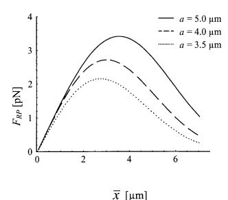
FIGURE 3 Numerical calculations of optical trap force,  $F_{\rm RP}$  (transverse force component), as a function of particle off-centering,  $\bar{x}$ , for beads of different sizes. The computations are performed for the trap configuration used in experiments and an applied laser power of 5 mW. The wavelength of the incident beam is 514 nm in air; the beam waist is 4.15  $\mu$ m.
