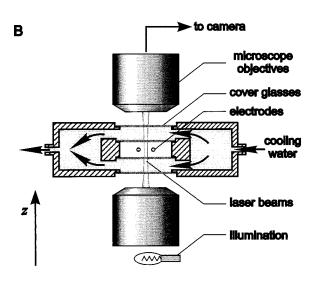
FIGURE 1 A schematic sketch of the experimental chamber. (A) Horizontal section: the cooling water cycle includes a cryothermostat. (B) Cross section: the optical trap is realized by two contrapropagating laser beams focused on the working cell by the two objectives.
