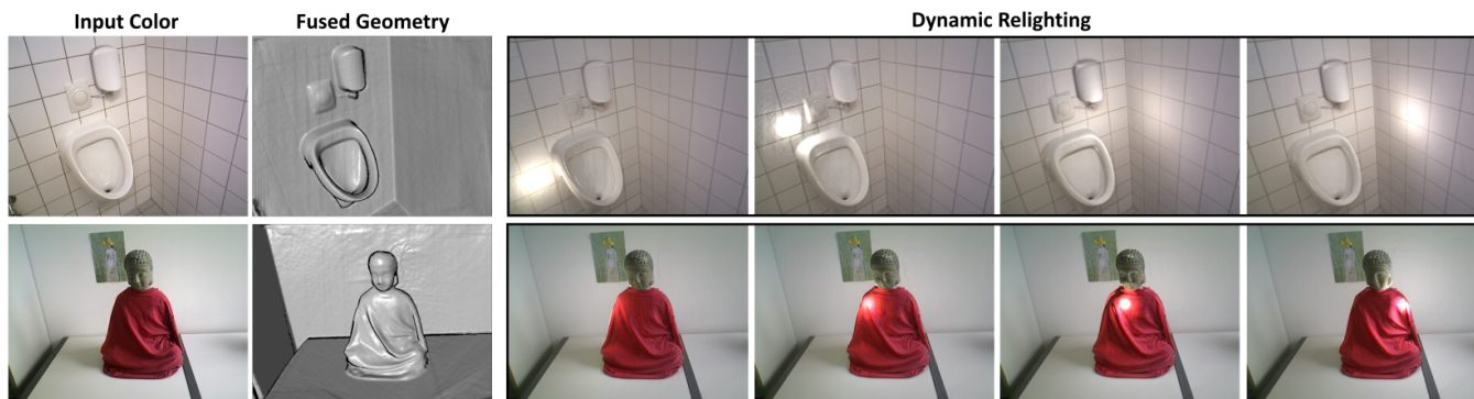
Figure 12: Dynamic geometry-based relighting. A virtual shading image is generated by rendering the scene geometry under a new light source. The resulting shading map is blended with the shading layer before recombining it with the reflectance to obtain a relighting effect.
