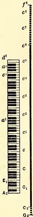
FIG. 13. The Series of Auditory Qualities. The keyboard of a grand piano extends from the A_2 of 27.5 vs. to the c^5 of 4224 vs. The smaller piano keyboard ranges between the C_1 of 33 vs. and the a^4 of 3520 vs. Helmholtz' lower limit of orchestral music is the E_1 of 41.25 vs. (double bass); his higher limit, the a^5 of 4752 vs. (piccolo flute). The organ has a range of 9 octaves: C_2 (16.5 vs.) to c^6 (8448 vs.). The highest note of the violin is the e^4 (2640 vs.). The range of audition is, approximately, from the G_3 of 12.35 vs. to the f^8 of 45056 vs.
