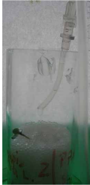
Figure 13: Fluid supply I: water dripping from end of Heidelberger Verlängerung washed away the plant and disturbed the packing.
