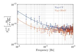
FIG. 3. Spectral density of consecutive measurements of  $\Delta g$  with  $V_{\rm TM}{=}1$  V and 20 mV. A combined fit to the background and  $V_{\rm TM}$ -dependent component is shown with continuous curves.
