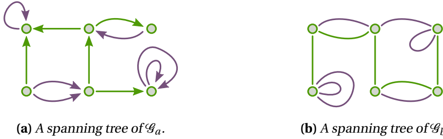
Figure 4.6: Examples of spanning trees for the graphs from figure 2.1. The spanning trees are depicted in green, their chords are colored violet.
