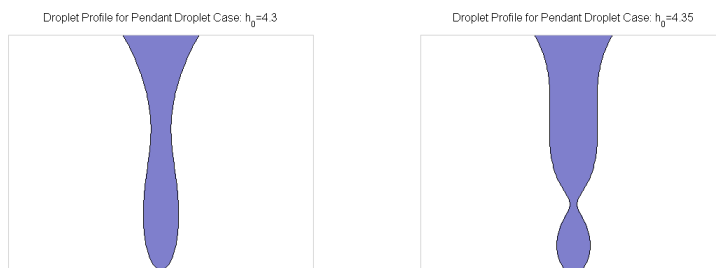
(a) Shortly before bifurcation. h_0 = 4.30 (units of capillary length) (b) Shortly after bifurcation. h_0 = 4.35 (units of capillary length)
