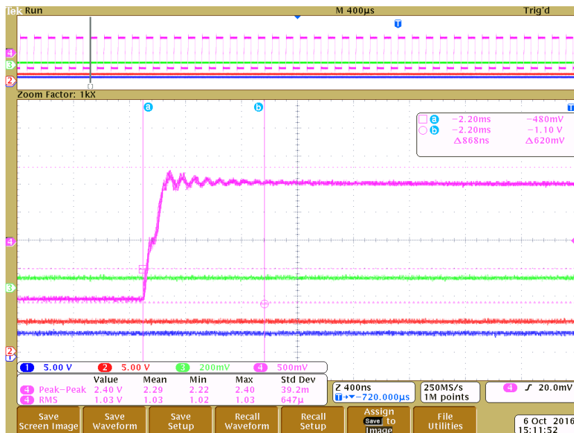
Fig. 19 Overshoot from the RP output. Rectangular signal at 10 kHz.
