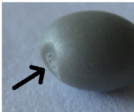
Figure 2.4: Imperfection of a plastic injection molded particle.
